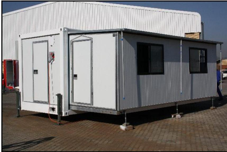
*Ablution container system with only one side extended*
